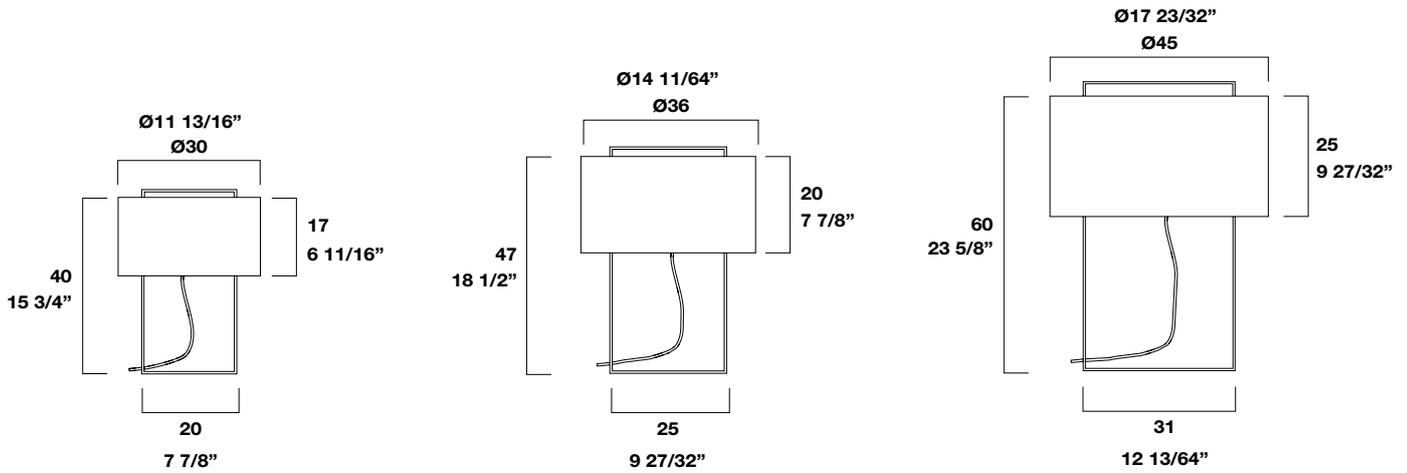
**Table giving ambient light. Cylindrical shade in black or white chintz fabric and new shades with fabrics of prestigious Kvadrat brand: coral, grey, green. Upper diffuser in perforated metal sheet enamelled white. Metal structure in 5x5 mm. square bar, enamelled black or white. Switching by means of on/off switch located in the electrical cable for the Lewit m40 version, and in the lamp-holder for the Lewit m47 and Lewit m60 versions.**
